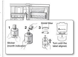
Once you have completed this process, hold the lce Off button simultaneously for 3 seconds to reset the filter schedule.
