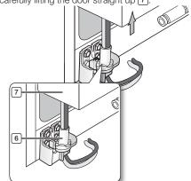
Be careful not to pinch the water tubing and wire harness on the door.
