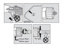
After connecting the water supply to the water filter, turn your main water supply back on and Dispense about 3L to clear and prime the water filter
