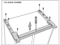
Remove hinge screws 3 and the ground screw
