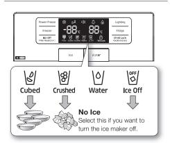
When Ice Off blinks on the display panel, reinsert the bucket and/or make sure it's installed properly.
