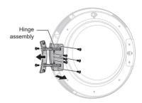
3 Remove the 3 screws from the door latch assembly which is fixed between the door and the hinge assembly and then remove the screw which is fixed on the door hook.
