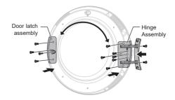
Remove the door catch from the appliance frame by removing 2 screws and then assemble them on the opposite side.
