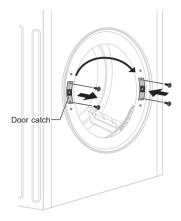
7 Install the door with the screws removed in step 1 and then check the door closes properly.
