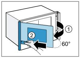
To loosen the panel, close the appliance door ① and at the same time press the fastening element on the appliance door down and towards the panel ②.
