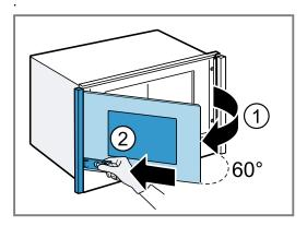
To loosen the panel, close the appliance door ① and at the same time press the fastening element on the appliance door down and towards the panel ②.
