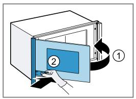
There may be noises when the panels are removed.3. Take hold of the panel on the side without the door hinges using both hands and remove it.
