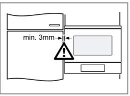
There must be an air gap of at least 3 mm between the appliance and adjacent cabinets.
