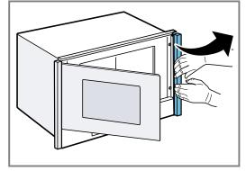
4. If the fastening elements have become loose when removing the panels, reattach them. Hook in the fastening element at the bottom and press down at the top until it is in place.
