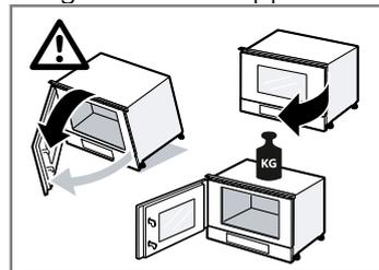
1. Open the appliance door 60° ① and slide a fastening element directly above the control panel between the appliance door and the control panel ②
