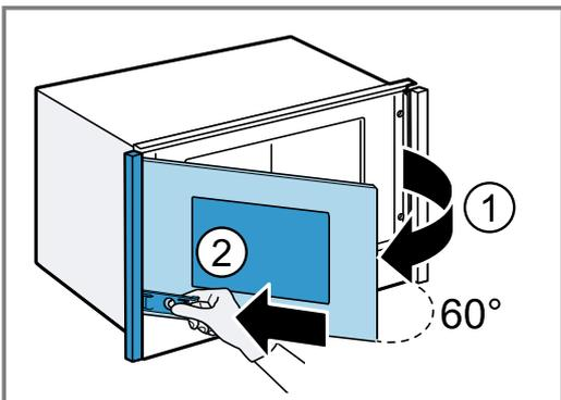
2. To loosen the panel, close the appliance door ① and at the same time press the fastening element on the appliance door down and towards the panel ②.
