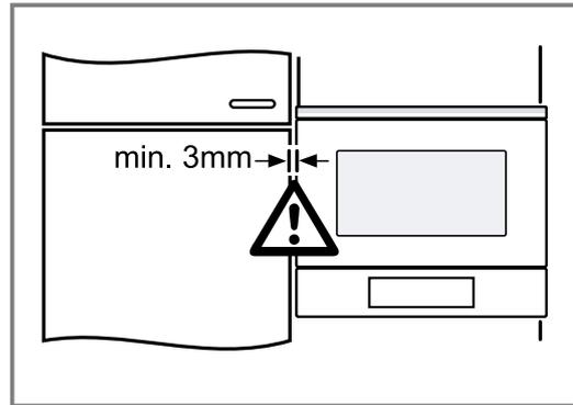
There must be an air gap of at least 3 mm between the appliance and adjacent cabinets.
