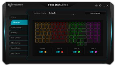
The keyboard backlight is divided into four zones, which you can turn on or off independently. In each zone, you can choose a custom color from the color square. Click the slider under each zone to turn the backlight on or off for that zone.
