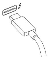
Type-C port is reversable; connectors may be inserted with either side up.
