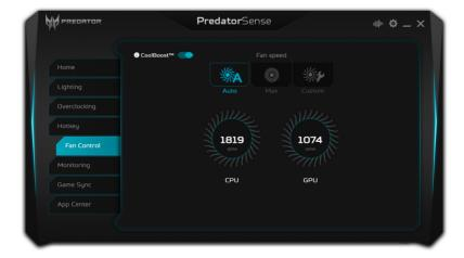
Activate **CoolBoost™** to increase fan speed beyond the normal maximum, enhancing cooling power when the system is under heavy use.
