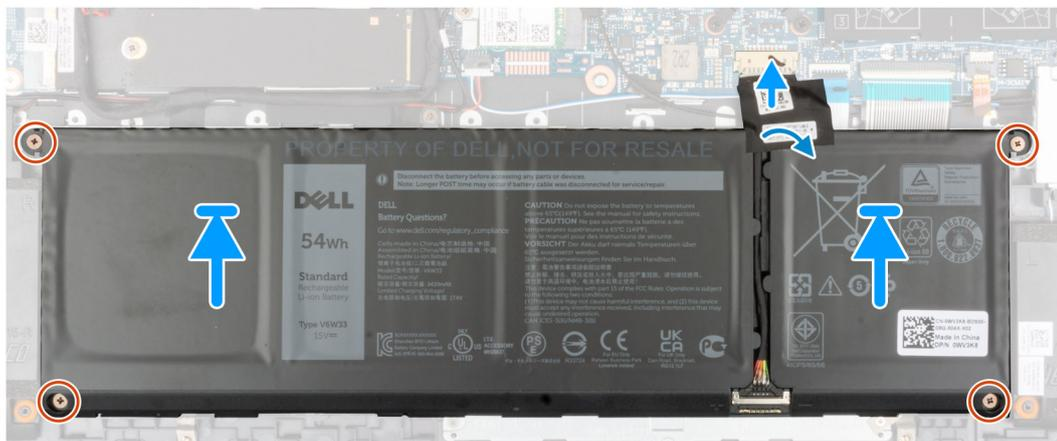
1. Using the alignment posts, place the 4-cell battery on the palm-rest and keyboard assembly.
