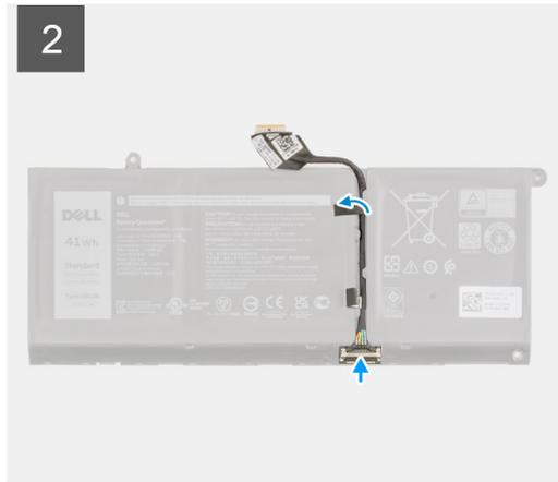
1. Align and place the battery cable on the battery.
