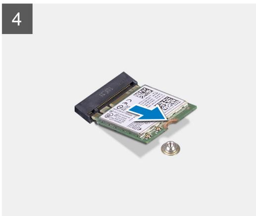
1. Remove the screw (M2x3) that secures the wireless-card bracket to the wireless card and system board.
