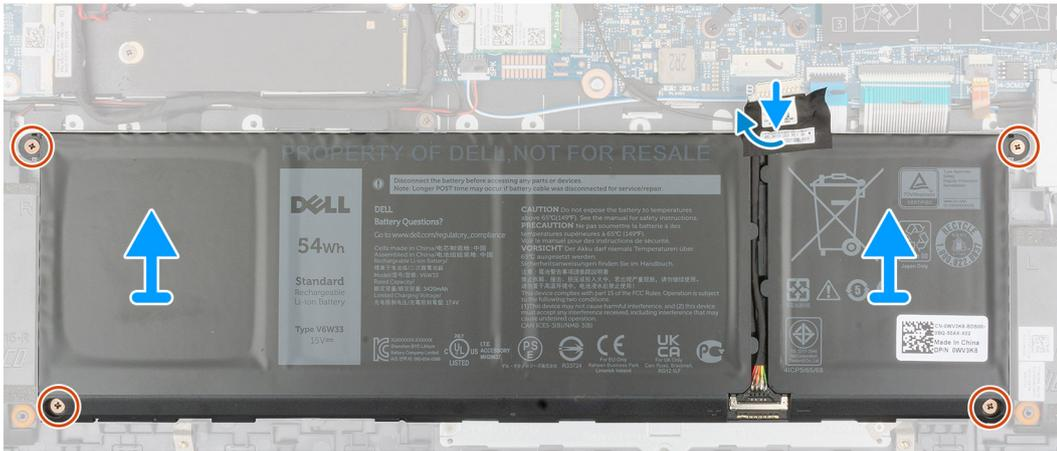
1. Peel the tape that secures the battery cable to the system board.
