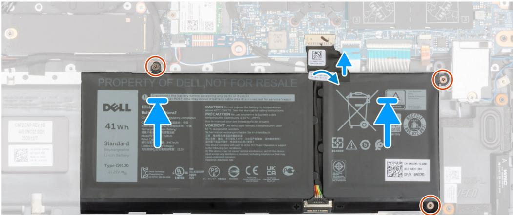
1. Using the alignment posts, place the 3-cell battery on the palm-rest and keyboard assembly.
