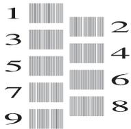
6. For the “A” pattern, swipe up or down or press ▲ or ▼ to display the number of the test print with the least visible vertical stripes (1-9), and then press it (in the example, number 6 is the best choice). Press [OK]. Repeat this step for the rest of the patterns.
