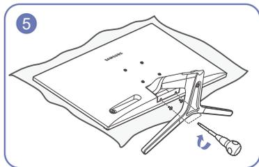
Fasten the screws at the bottom of the stand neck.
