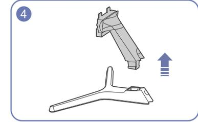
Remove the stand neck from the stand base by pulling it in the direction of the arrow as shown in the figure.
