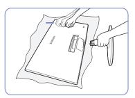
While holding the stand neck with one hand, pound the other fisted hand down onto the top of the stand base in the direction of the arrow to detach the stand base.
