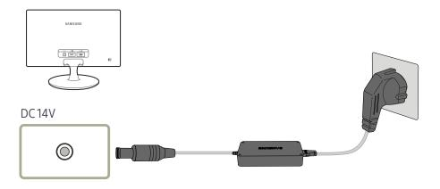
The input voltage is switched automatically.
