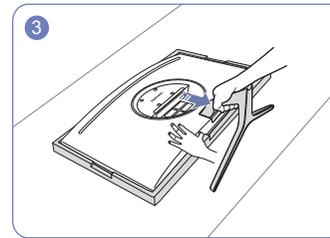
Press the lower part of the monitor with one hand, and pull the stand with the other hand in the direction of the arrow as shown in the figure.
