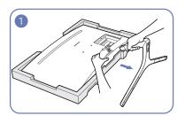
Place the protective Styrofoam (cushion) included in the package on the floor and place the product facing down on the Styrofoam, as shown in the image. If Styrofoam is unavailable, use a thick sitting mat. While holding the monitor with one hand, pull the stand neck with your other hand to in detach the stand as shown in the figure.
