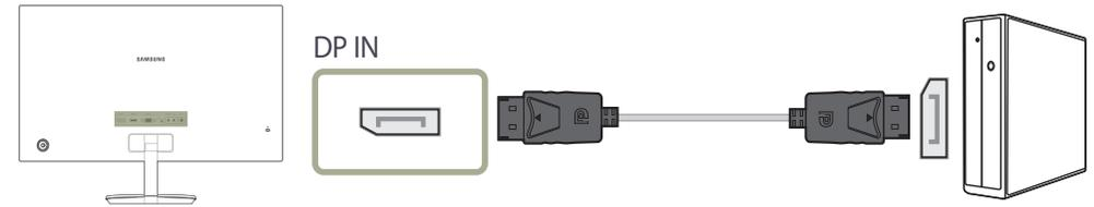
— A DP cable shorter under 1.5 m in length is recommended. Using a cable longer than 1.5 m can affect the picture quality.
