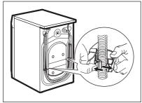
**10.** Remove the three bolts by using the spanner supplied with the appliance.
