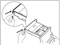
Remove the insert for the softener and, if inserted, the container for liquid detergent.
