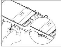
4. Press the catch on the back as indicated in the picture and lift up the top cover to remove it.
