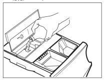
Gently pour only liquid softener in the AutoDose fabric softener tankFill up to the maximum indicated
