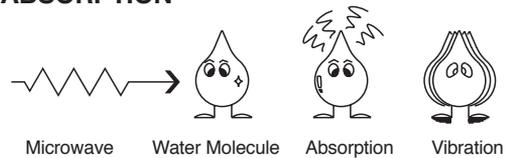
The microwaves cause the water molecules to vibrate which causes **FRICTION**, i.e. **HEAT**. This heat then cooks the food. Microwaves are also attracted to fat and sugar particles, and foods high in these will cook more quickly.
