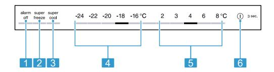
alarm off switches the warning signal off.
