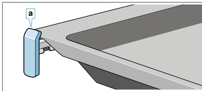
The pull-out rails lock in place when they are fully pulled out. This makes it easy to place the accessories in position. To unlock, push the pull-out rails back into the cooking compartment with a certain amount of force.
