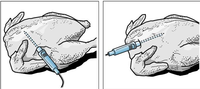
**Turning the food:** If you wish to turn the food, do not remove the meat probe. Once you have turned the food, check that the meat probe is correctly positioned in the food.
