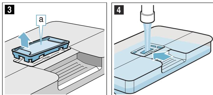
7. Reinsert the cover **a** into the opening in the water tank.
