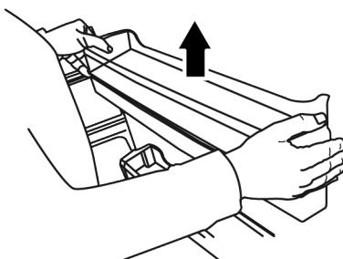
2. Hold both sides of the water tank and remove at 45° angle.
