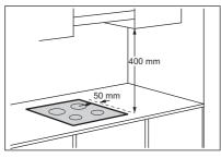
If a furniture unit is installed at a distance of 400 mm above the hob, there must be a minimum safety distance of 50 mm to the left or right from the edge of the hob.
