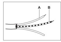
Connect the green and yellow (earth) wire to the terminal which is marked with the letter 'E', or the earth symbol , or coloured green and
