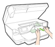
**c.** Move the carriage to the left, locate any jammed paper inside the printer on the right side of the carriage, free any paper scraps or wrinkled paper, and pull the paper towards you through the front of the printer.
