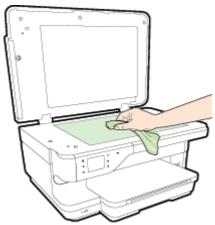
**CAUTION:** Do not spray the glass cleaner directly on the scanner glass. If too much glass cleaner is applied, the cleaner could leak under the scanner glass and damage the scanner.
