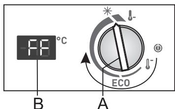
We recommend using this setting before cleaning the appliance or 24 hours before inserting a large amount of food. Activating this function will make sure the food is cooled or frozen faster to retain vitamins, minerals, nutrients, and flavour, and to extend its freshness.
