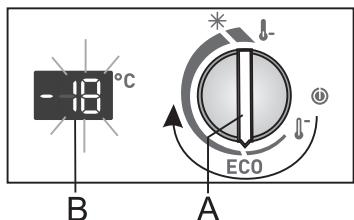
A signal will be given when the temperature in the appliance is too high. The set temperature shown in the display and, if present, the LED lighting will flash.
