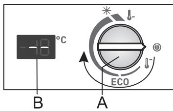
**Switching on:** To switch on: rotate the **A** dial clockwise.
