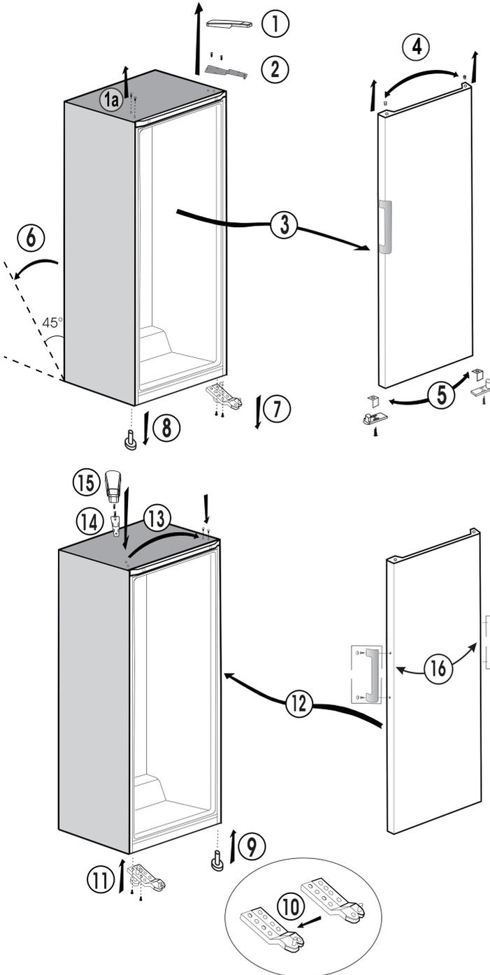
1. Remove the plastic cover of the top hinge.
