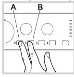
To start the programme press buttons **A** and **B** simultaneously for 5 seconds (see figure).
