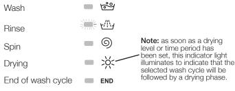
**Note:** during the "Drain" phase, the indicator light corresponding to the "Spin" cycle phase will illuminate.
