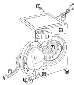
1 Transit bolts 2 Power plug 3 Drawer 4 Control panel 5 Drum 6 Door 7 Drain hose 8 Drain plug 9 Drain pump filter 10 Cover cap (Location may vary depending on products) 11 Adjustable feet
