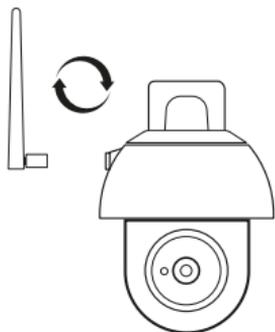
Screw antenna into rear of camera.
