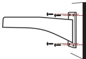
Hang the camera on the 4 screws, then fasten 4 screws by using hex key.
