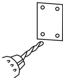
Drill the mounting holes by using the alignment paper.
