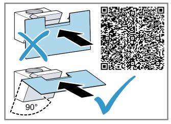
2. Insert the brackets for the filter cover into the openings on the appliance and lock into place.
