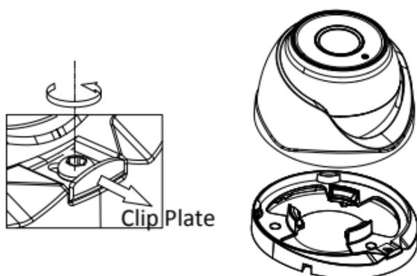
Figure 2-8 Remove the Clip Plate
