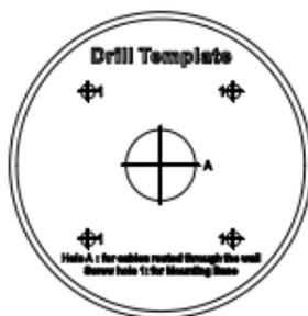
Figure 2-12 Drill Template of the Junction Box
