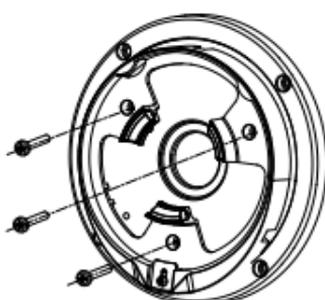
Figure 2-13 Secure Screws on Junction Box's Cover
