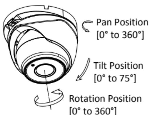
Figure 2-11 3-axis Adjustment
