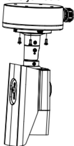
Figure 2-4 Fix the Camera with the Gang Box
