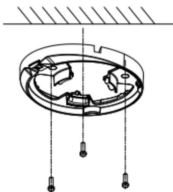
Figure 2-9 Fix the Mounting Base on the Ceiling
