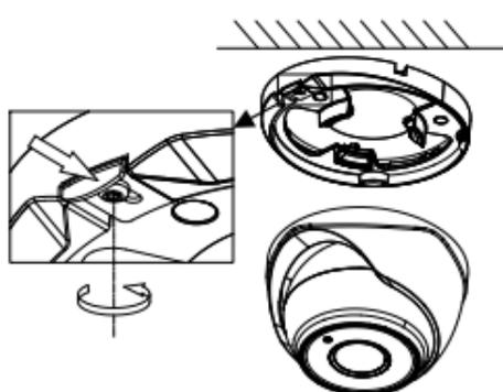
Figure 2-10 Install the Turret Camera
