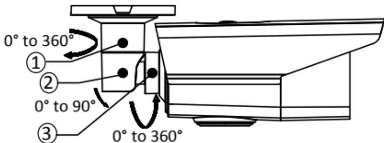
Figure 2-3 3-axis Adjustment
