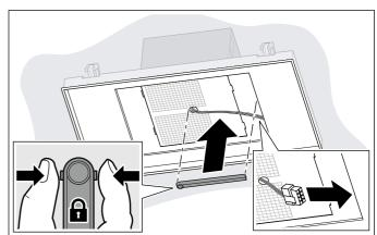
Press together the cable duct at the sides, attach and click into place.
