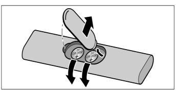
3. Correctly insert the new batteries (3 V CR 2032).
