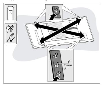
Carefully tighten screws in succession until the appliance is flush-mounted on the ceiling.
