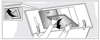
4. Take the metal grease filter out of the holder.
