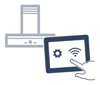
If the extractor hood has successfully connected, it will automatically connect to the Home Connect app. LED 3 and LED 7 will flash.
