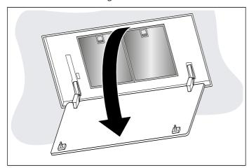
Open the lock.Note: To avoid causing damage, do not bend the metal grease filter.
