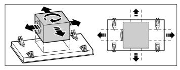
5. Push the fan box to the side and connect the power supply.
