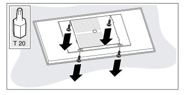
**4.** Turn the fan box into the correct position according to the installation situation.
