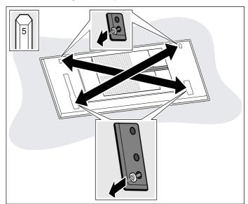
8. Push the removal slide inwards to loosen the mounting brackets.
