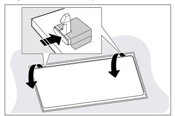
Open the filter cover fully and without pulling on it.
