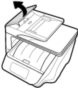
2. Pull any jammed paper out of the rollers.
