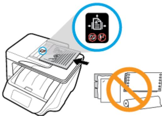
2. Slide the paper-width guides inward until they stop at the left and right edges of the paper.
