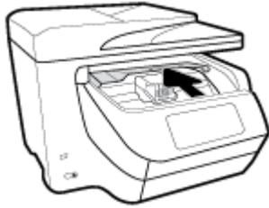
2. If the print carriage is not obstructed, move the print carriage to the far right of the printer and remove the jammed paper.
