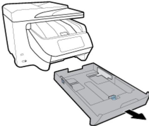
2. Check the gap in the printer where the input tray was. Reach into the gap and remove the jammed paper.
