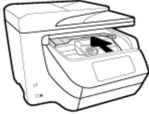
3. Press the front of the cartridge to release it, and then remove it from the slot.
