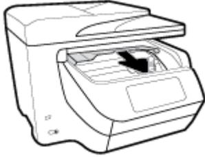
6. Remove Tray 1 by pulling it out from the printer.
