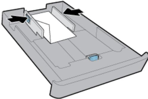
5. Make sure the stack of envelopes does not exceed the stack height marking on the left paper-width guide.
