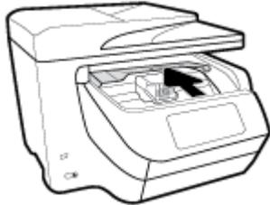
2. Open the inside cover by lifting and moving it towards you.
