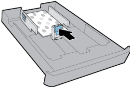
7. Check the input tray area underneath the printer. If there is paper, remove the paper.
