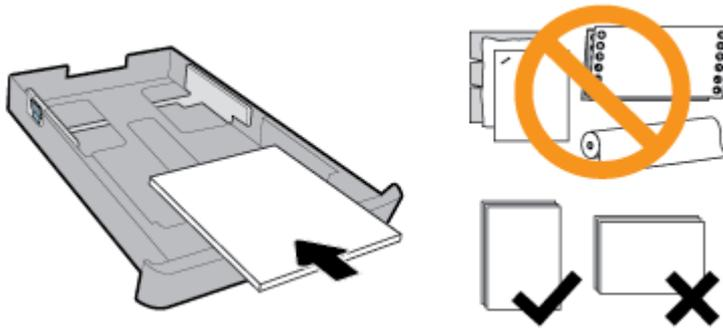
Make sure the stack of paper is aligned with the appropriate paper size lines on the front of the tray. In addition, make sure the stack of paper does not exceed the stack height marking on the right edge of the tray.
