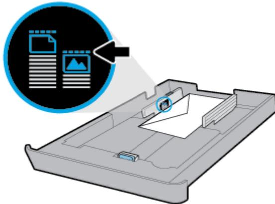
6. Adjust the paper-length guide until it touches the edge of the stack of envelopes.
