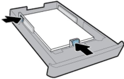
5. Check the Tray 2 area underneath the printer. If there is paper, remove the paper.
