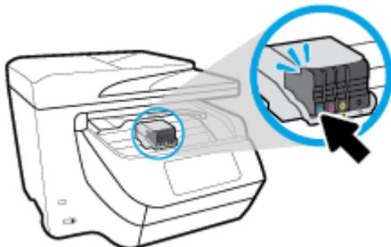
Make sure that the color-coded letter on the cartridge matches that on the slot.
