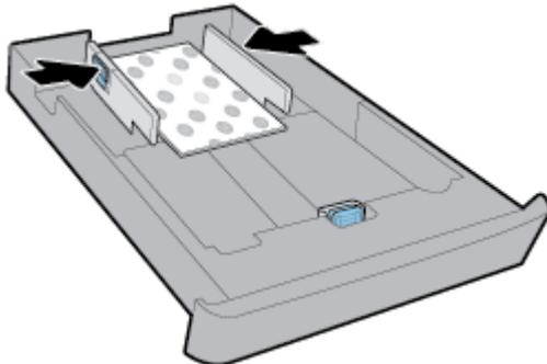
5. Make sure the stack of paper does not exceed the stack height marking on the left paper-width guide.
