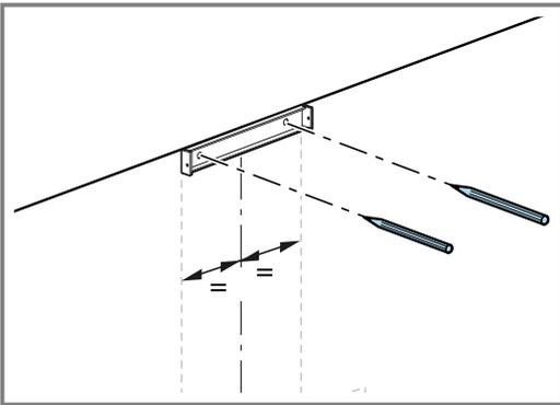
Measure and mark the drill holes for the fastening screws.
