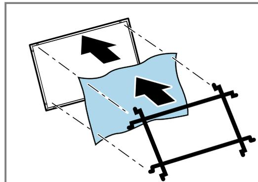
3. Use the grid to secure the odour filter to the outer holes.
