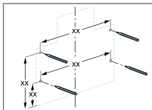
The bottom edge of the appliance is identical to the lower edge of the drilling template.
