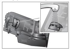
■ Thoroughly clean the connecting nozzles of the brewing unit.
