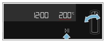
The appliance will start heating. The ▷|| LED will be lit. The length of the bar on the temperature indicator gradually increases.
