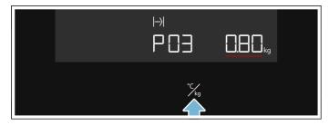
**4.** Use the rotary selector to set the weight to 1 kg. The appliance automatically sets the right cooking time for that weight.
