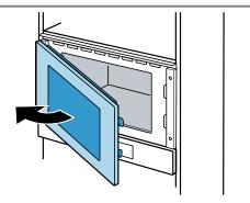
**4.** Screw the appliance to the unit on the opposite side to the hinges.
