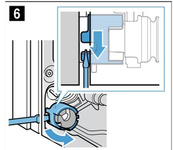
**Removing and installing the door panels**
