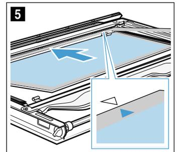
5. Push down on the intermediate panel around **b**, slide the holder **c** in at an angle and push down until it clicks into place (Fig. 6). The holder has been inserted (Fig. 7).
