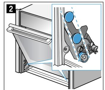
2. Rotate the door handle upwards slightly **a** (fig. 3). The appliance door will slide the short distance remaining to the bottom **b** (fig. 3).
