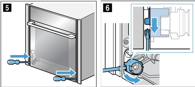
**Removing and installing the door panels**
