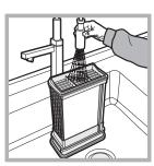
Step 3 Flush the condenser, from the rear with water, to remove any fluff deposits.
