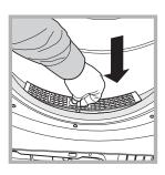
Step 5 Refit the filter – Never run the dryer without a filter.
