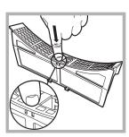
Step 3 Open the filter by releasing the clip.
