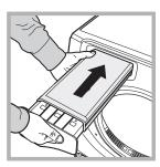
Step 3 Refit the Water Container ensuring that it is pushed fully back into position.
