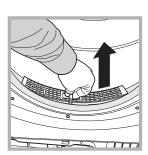
Pull out the filter (using the two finger grips).
