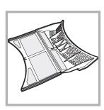
Step 4 Clean any fluff deposits from the inside surface of the filter mesh.
