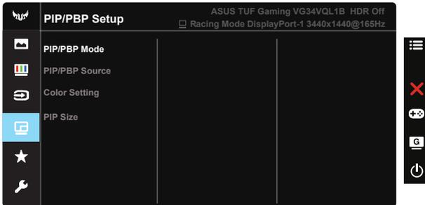
By activating this function, this monitor displays two pictures, three pictures or four pictures for any video source.
