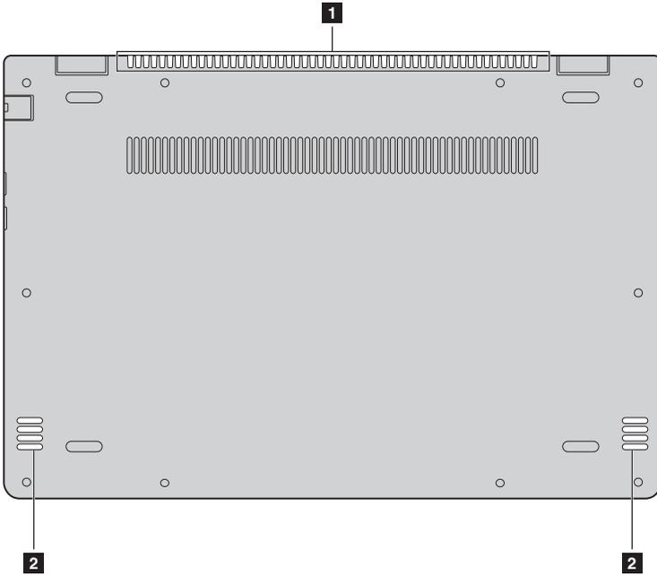
**1 Ventilation slots** Dissipate internal heat.
