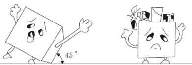
1. The appliance should not be tilted more than 45 degrees when you move it. Do not use force on any part such as the condenser, the door or handle. They could distort and affect the operation of the refrigerator. Ensure ALL packaging is removed before installation
