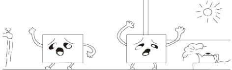
3. The appliance should not be installed near external heat sources eg direct sunshine - or external moisture sources.
