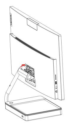
6. Slightly press the hinge cover until it snaps into position.
