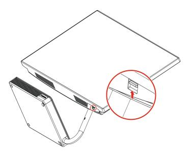
4. Pull the storage drive and the bracket out.
