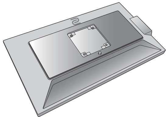
Orient and align the stand arm with the monitor (1), push them together until they click and lock into place (2).
