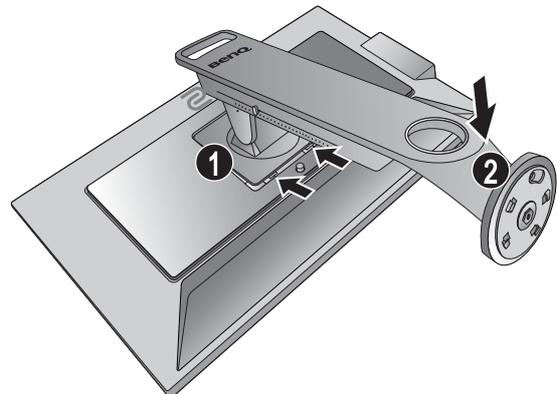
Orient and align the stand base socket with the end of the stand arm. Make sure to align the arrow on the end of the stand to the one on the monitor base.
