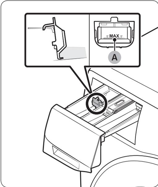
First insert the provided liquid detergent container in the **II main-wash compartment**. Then, apply liquid detergent to the container below the marked **max line (A)**.
