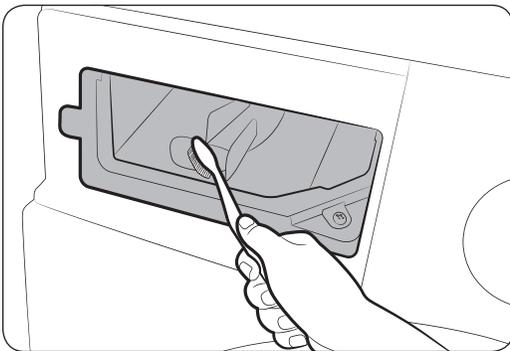
1. While holding down the **release lever** inside the drawer, slide open the drawer.
