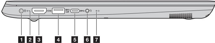
**1 AC power adapter jack** Connects to the AC power adapter.
