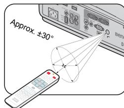
Make sure that there are no obstacles between the remote control and the IR sensor on the projector that might obstruct the infra-red beam.
