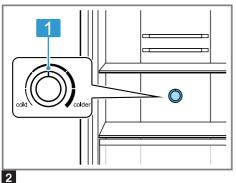
The temperature controller sets the temperature.
