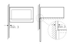
Measurements in mm
