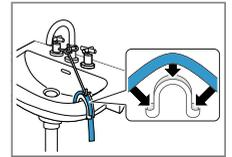
Drainage into a plastic pipe with rubber sleeve.
