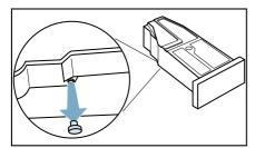
Turn the condensation container 180° again and insert the stopper into the recess in the top of the condensation container.
