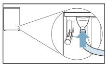
Secure the other side of the drain hose using the remaining accessories, depending on the connection situation.
