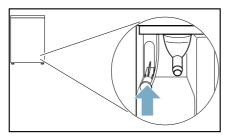
5. Push the drain hose as far as it will go onto the uncovered socket.
