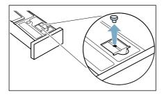
Turn the condensation container 180° onto its underside and insert the stopper.
