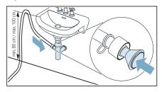
The connection point must be secured using a hose clamp (12-22 mm clamping range, available from specialist retailers).
