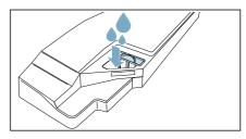
**Note:** Hold the full condensation container horizontally at all times so that no liquid spills out.
