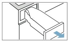
Push the condensation container back into the appliance until you feel it lock into place.
