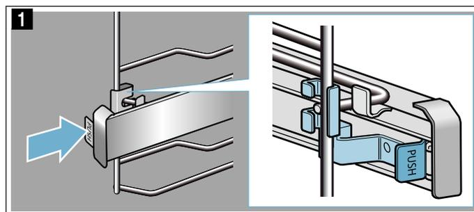
2. Keep the "PUSH" tab pushed back and swing the rail out (fig. 2).
