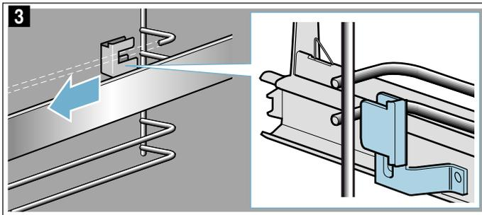
4. Remove the pull-out rail (fig. 4).
