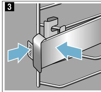
4. Release the "PUSH" tab; the retainer will hook into place (fig. 4). Then pull the rail out as far as it will go and slide it back in.
