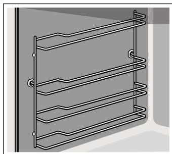
1. Lift the rail slightly at the front **a** and detach it **b** (fig. **1**).
