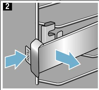
3. Pull the rail out towards you until the retainer at the back unhooks (fig. 3).
