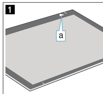
2. Check the fit of the four spacers and two seals on the intermediate panel:
