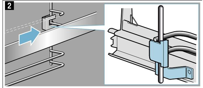
3. Push on the "PUSH" tab and swing the rail in so that the retainer ends up between the two bars (fig. 3).
