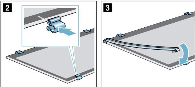
3. Insert the intermediate panel with the seals and spacers. The arrow on the intermediate panel must line up with the arrow on the frame (Fig. 4).
