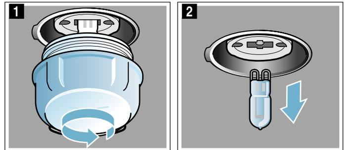
4. Screw the glass cover back on. Depending on the appliance model, the glass cover may have a sealing ring. If the glass cover has a sealing ring, put it back in place before screwing the cover back on.
