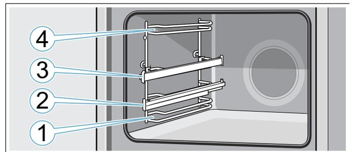
Always insert accessories between the two guide rods for the shelf position.
