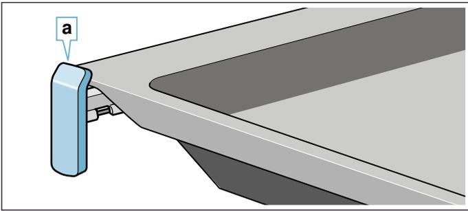
The pull-out rails lock in place when they are fully pulled out. This makes it easy to place the accessories in position. To unlock the pull-out rails, use a little force to push them back into the cooking compartment.
