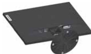
Step 3: Remove the base and stand from the monitor, refer to "Detaching the monitor base and stand" on page 2-11".
