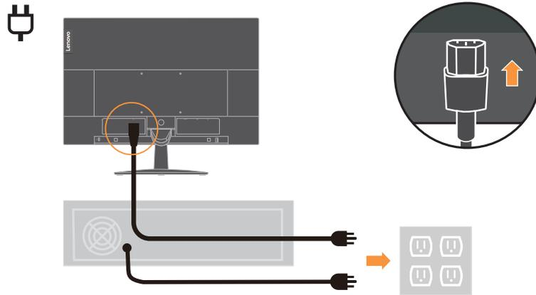
7. Connect the cables with cable clip.
