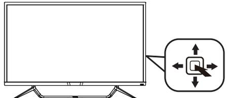
To access the OSD menu on this Philips Display simply use the single toggle button on the backside of the Display bezel. The single button operates like a joystick. To move the cursor, simply toggle the button in four directions. Press the button to select desired option.
